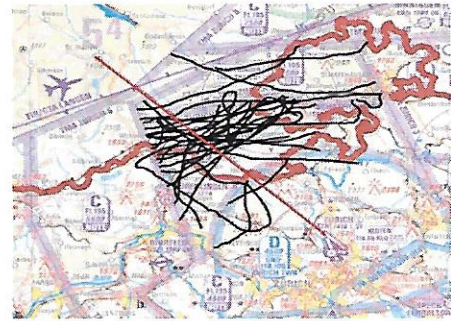
Red line = ILS 14 in LSZH, black lines = Flighttracks inside TMA 2009 without clearance
